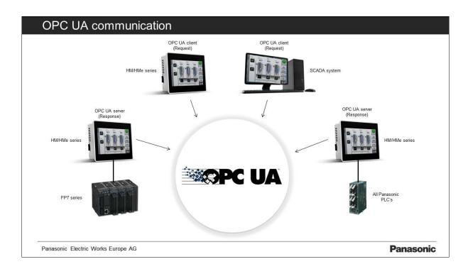
The key component of the Panasonic OPC UA mechanism is the touch terminal. If the touch terminal is used as the OPC UA server, the data points can be made available in the HMI with a defined semantic. Every OPC UA client can browse the tags in the HMI and use them for inter-machine data exchange. Another security feature is the access protection which can be added to variables/groups of variables/alarms/trends so that these items cannot be browsed or used by the OPC UA client.
