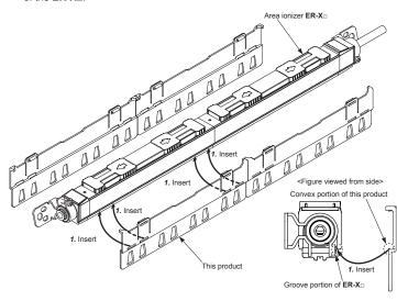
2. Press down on the latches in 2 locations on the upper portion of this product against the ER-X□. When installing, align the lines of this product and the ER-X□ as shown in the figure below.
