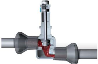
Large valve with controlled actuating drive
