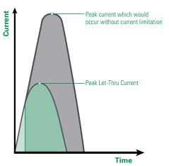
Figure 6 - Current limiting effect of fuses
