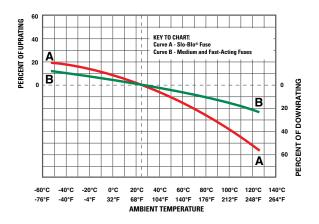
Figure 2 – Fuse Rerating Curve
