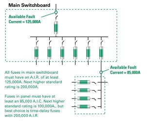
Figure 1 – Interrupting Rating Requirements per NEC
