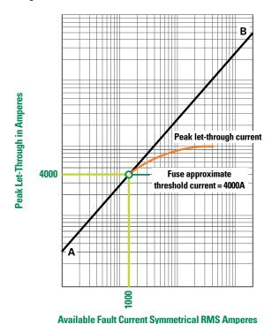
Figure 19 – Determining Threshold Current from Peak Let-through Chart
