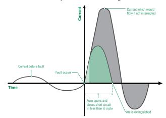
Figure 13 - Current-limiting Fuse
