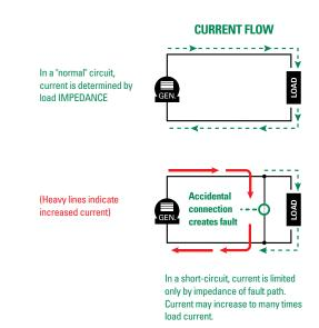
Figure 16 – Current Flow in Normal and Short Circuit Situations
