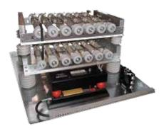
Neutral-Grounding Resistors (NGRs) are used to ground power systems by inserting a resistor between the system neutral and ground. This lowers the prospective ground-fault current to a predetermined value.
